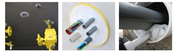
**VISCOSEALANT:** waterproofing cable and pipe penetrations. Left picture: sealing penetrations at vault system for control valves. Middle picture: multiple cables in one sleeve. Right picture: viscous elastic behavior during filling: the viscous component is dominant during filling and allows for flow around and in between the pipes, while the elastic component takes over when the material is in place; therefore no dripping or running can occur.
